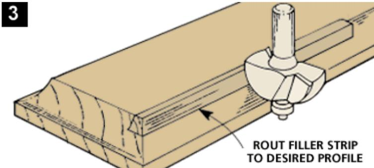
3. Now the original profile can be routed in the filler strip. (Hopefully without chipout this time.)
